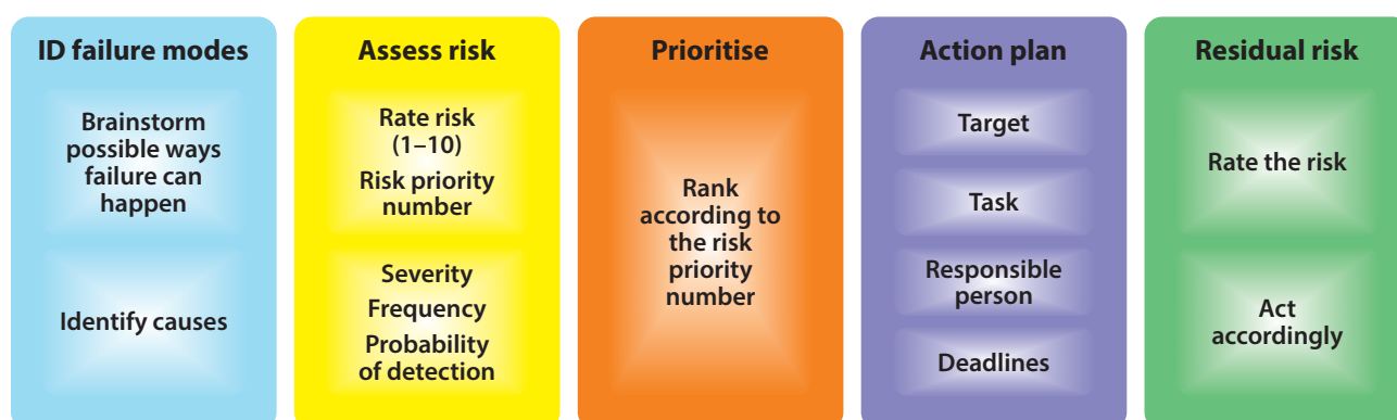
Figure 2.2. Failure mode effects and criticality analysis (FMECA)
